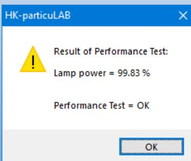
To check the performance of the laboratory device it is possible to make a performance test with a reference plate.
